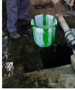
Fig.1. Flow rate calculation by bucket method
