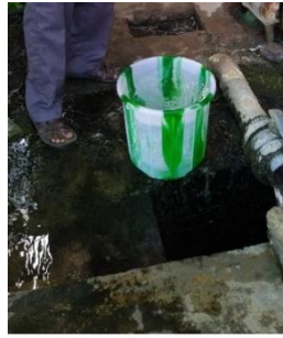
Fig.1. Flow rate calculation by bucket method
